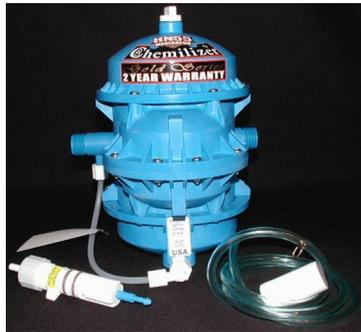
The Chemilizer pump motor has a diaphragm. This prevents wearing of the piston and the cylinder walls, which causes inaccuracies in metering, a major problem in low-flow systems. Minimum water flow required is 29 gal/day. 2-year factory warranty. Ship. Wt. 6 lbs.
