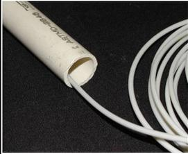
These cables are for use in preventing water line freeze-ups in areas with extended periods of low temperatures. Each combination of lengths and wattage below provides 5 watts / ft of cable, which is adequate to protect water lines down to 10 °F. For protection to zero Fahrenheit, install two cables into the line. All models listed are 120 V cables. **CAUTION:**
